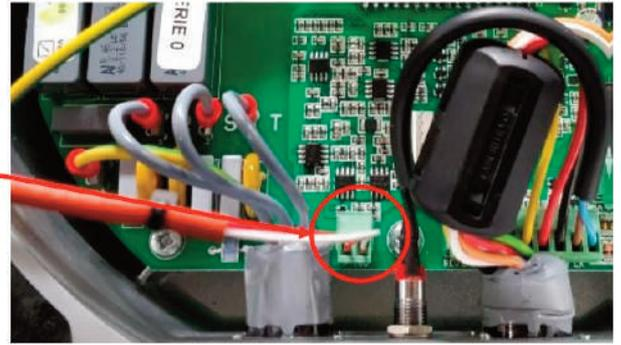
*INSERT THE GREEN CONNECTOR, WITH THE WHITE/RED WIRES, OF THE ENGINE TEMPERATURE SENSOR INTO THE SPECIAL CONNECTOR ON THE ELECTRONICS (AS POSITIONED IN THE FIGURE).*
