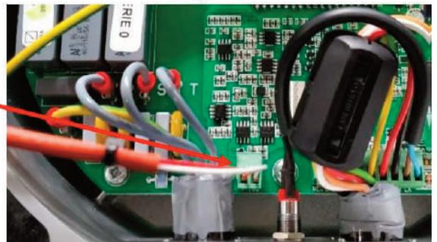
*DISCONNECT THE FASTONS ON THE ELECTRONICS OF THE MOTOR PHASES AND PT100*
