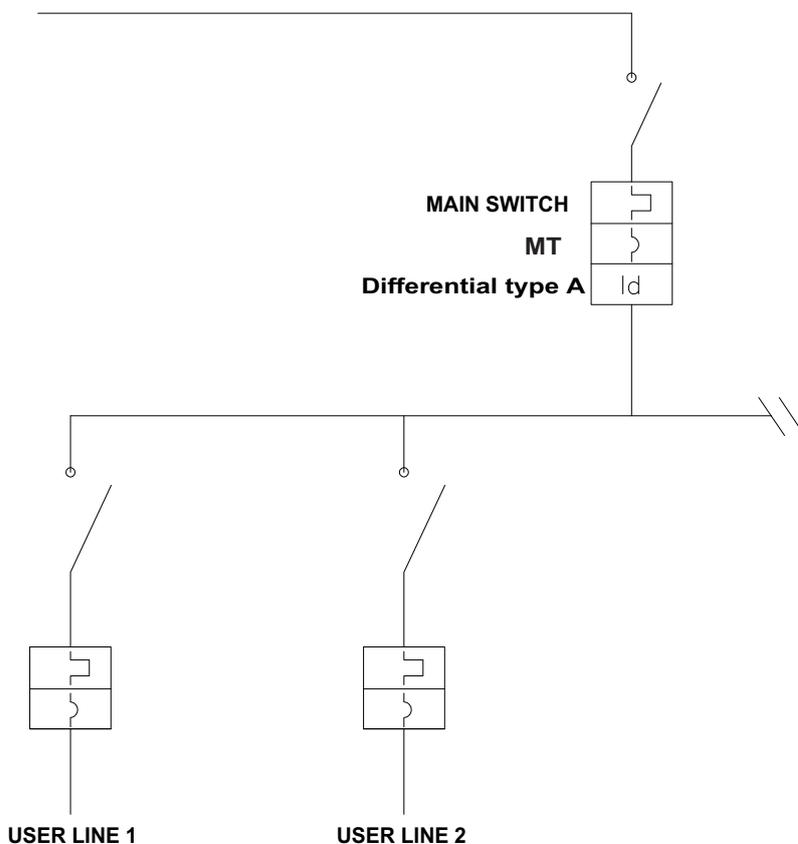
Dedicated line suitably protected with Magnetic-Thermal Switch and Differential Class A with a sensitivity of 300 mA.
