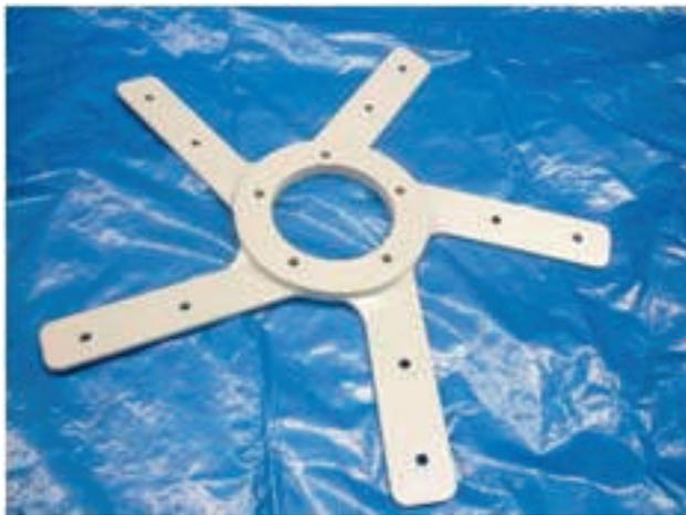
*Reinforced star blade holder folded + spacer*
