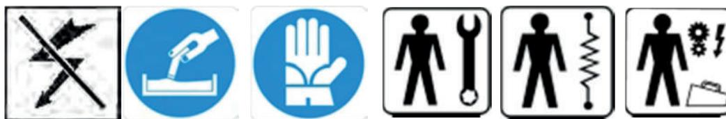
**Before doing any maintenance work, isolate the equipment from the power supply and shut off the water supply!**
